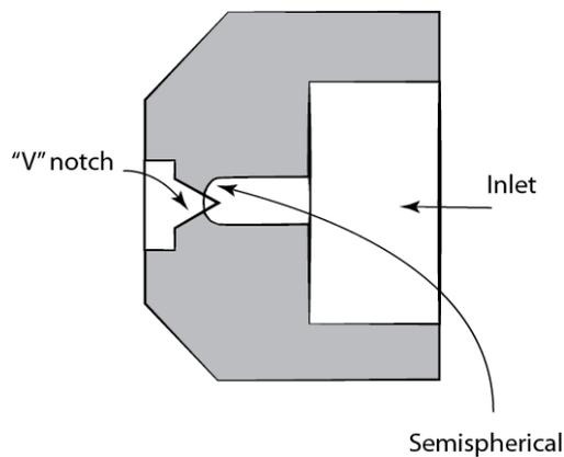
Figure 1 - Flat fan nozzle geometry
