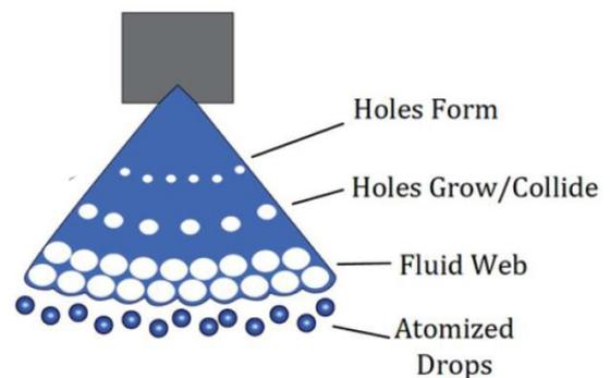
Figure 5 - Perforation breakup model
