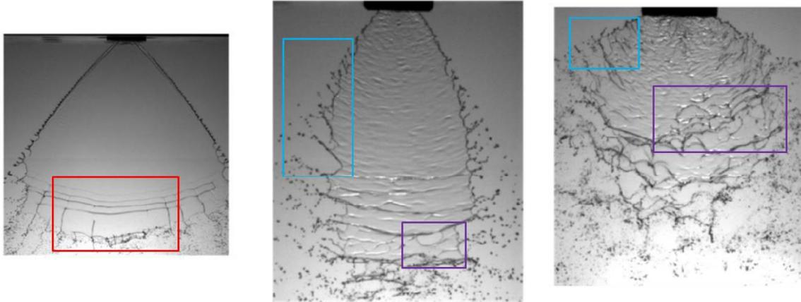
Figure 3 - Different break up mechanisms (wavy sheet - red) (rim - blue) and (perforation - purple)
