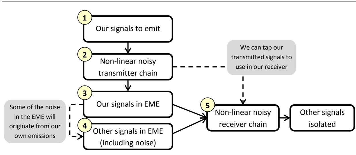
**Figure 2: Flow model for the challenge**
